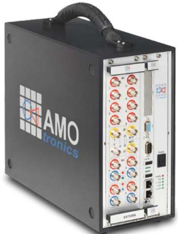
The **FlatSaturn** displayed above is the most compact housing option with up to 16 (BNC) or 48 (SMB) channels at different sampling rates. The small and rugged design makes it a popular portable instrument.
