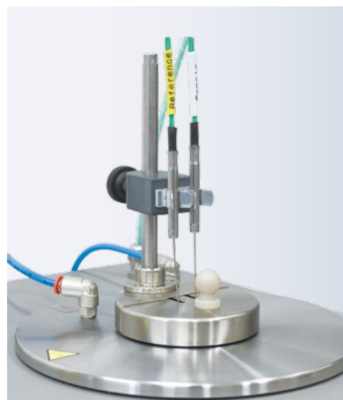
DTA 552-Ex – detail of the furnace
