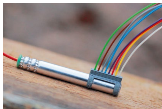
Detonation velocity measurement of a blasting cap
