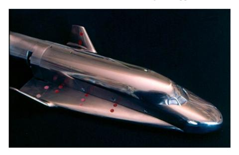
In addition to being equipped with numerous pressure sensors, heat flow sensors should be fitted above all on the underside and at critical points such as the fuselage nose and the leading edges of the wings. The equipment with pressure probes based on the very high-frequency PVDF sensors just developed by Müller und Platte, a forerunner of today's M60-3 model, as well as Kistler sensors could be easily solved.
