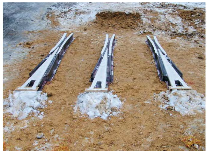
Application of the sheet explosive during railway frogs explosive hardening
