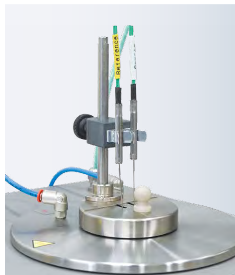
DTA 552-Ex – detail of the furnace
