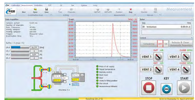
Measurement module with remote control section during data recording (after firing el. fuse-head)
