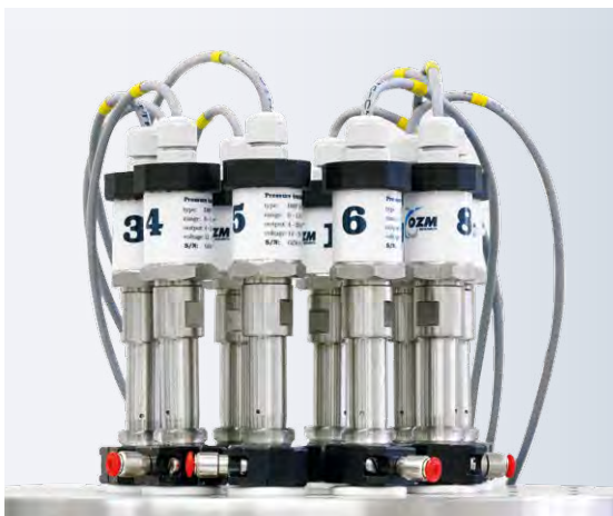
STABIL – pressure transducers during experiment
