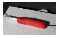
the plastic fiber optic cable with miniature holes created in its core. The Perforated Fiber Probe is simply placed perpendicular to the charge axis. The detonation wave generates sharp peaks on the light signal as it passes the holes and the detonation velocity is then determined from the distances between the holes and the corresponding peak times. Using this technique, detonation velocity of a single explosive charge can be measured by a single channel.
