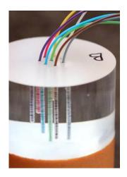
The glass fiber optic probes are small in diameter which allows better precision their placement compared to the plastic probes. Virtually single grain of explosive is captured by the probe which is useful in testing the smallest charges. Distances of more than 500 m between the explosive
