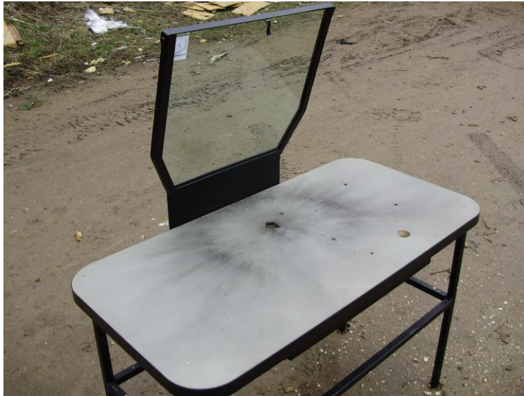
The pyrotechnic desk after explosion of 10 g of PBX (Semtex 1A) on the surface of the table.
