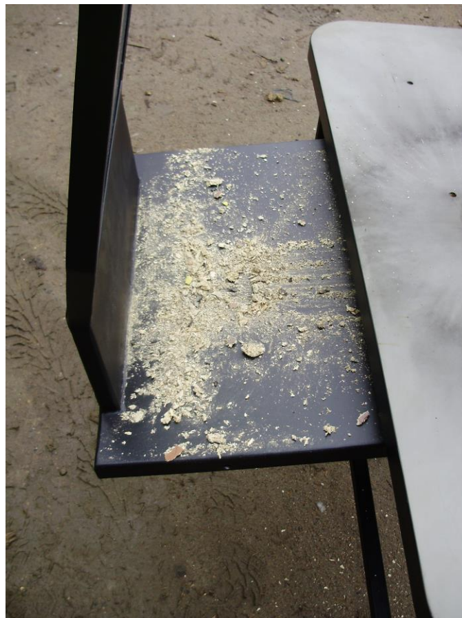
Fragments of the wooden board after explosion of 10 g PBX (Semtex 1A). The steel plate protects worker's legs against the fragments.
