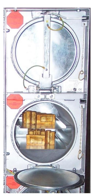
Storage modules have been designed and tested to **prevent transfer of explosion** (deflagration or detonation, action of shock wave, fragments or sharp flame) between modules. Modules are rectangular-shaped boxes with connecting points for mounting them together creating blocks with user-defined heights and lengths.
