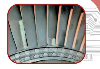
Remedial works due to cracks propagation on the walls of the combustion chamber. HPM nickel-chromium wire strain gages were installed using VPG HG-1 cement. Elongation cable routes are
