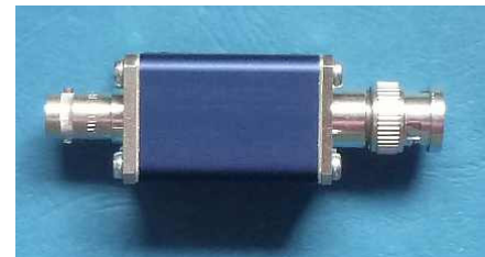
1 MHz filter for connecting the output cable to the recorder
