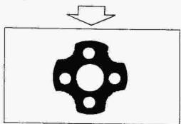
Withdraw the film. The pressure distribution is readily observable by the color density pattern formed on the C-Film.
