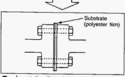
3. Insert the "sandwiched" film into the place to be measured and apply pressure.
