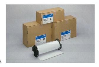
The UV-light measuring film can be equally prepared as the heat flux film Thermoscale or pressure measuring film Prescale. Cut by scissors it is placed on the body to be tested. Within the film are microcapsules and color developer which react to exposure to and stain the slide. The intensity of the colour is proportional to the amount of UV light.
