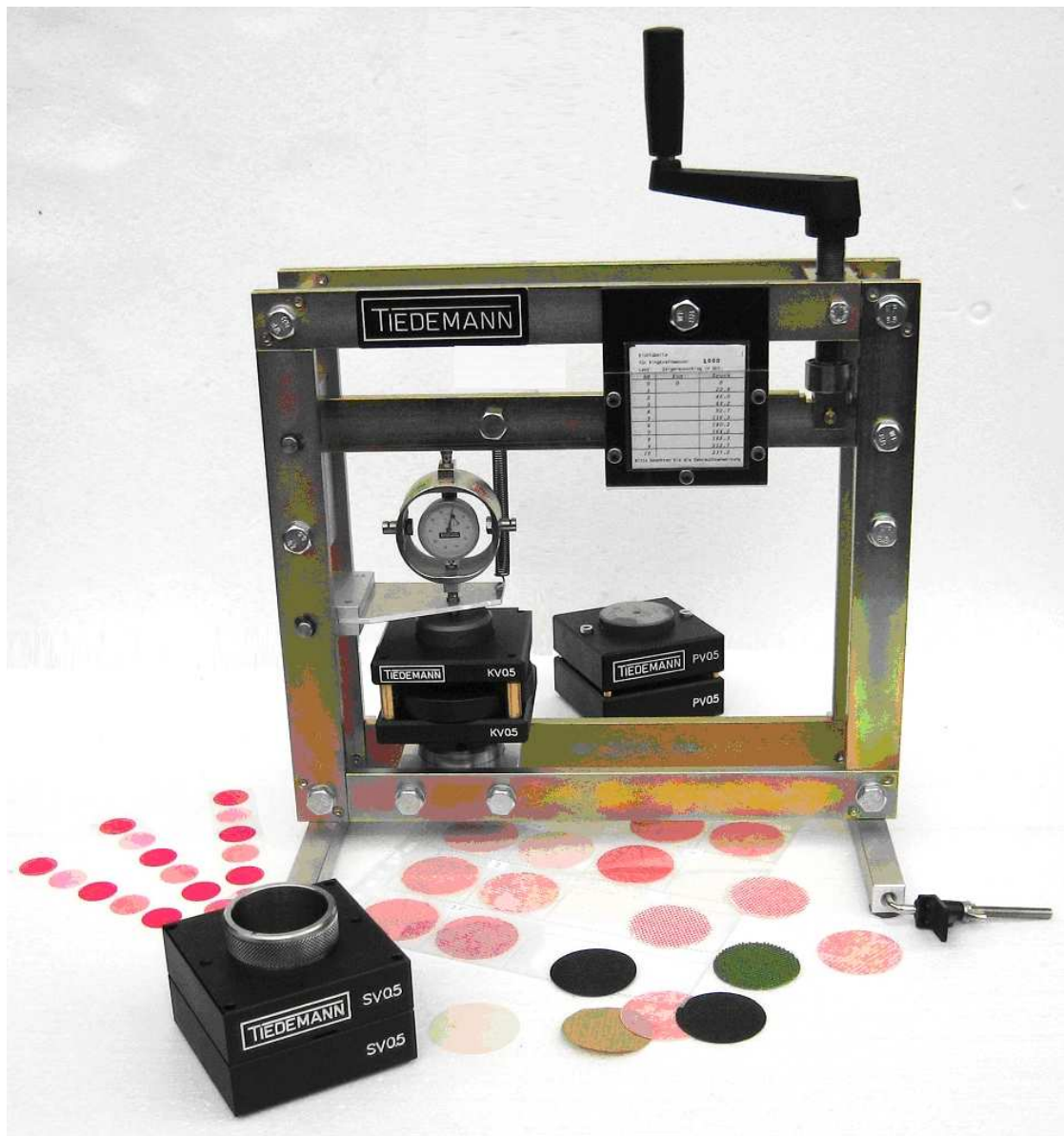
Calibration plunger in the compression device with dynamometer and additional tools
