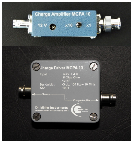
Charge Amplifier with Charge Driver in the principal experimental set up
