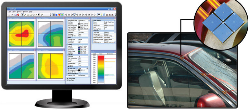
Tactilus Free Form ® sensors placed on a car door seal
