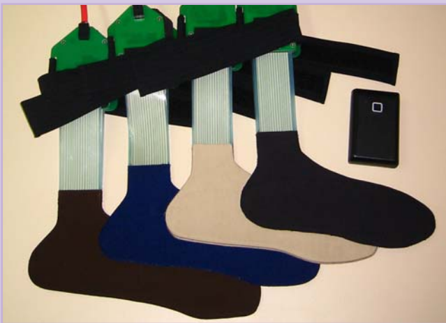
The Tactilus® foot insole sensor, to be inserted into shoe
