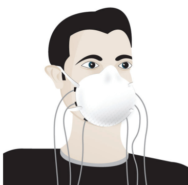
Example of Tactilus Free Form ® being used for face mask sealing pressure measurement
