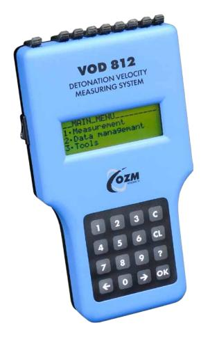
with an adjustable level of positive or negative triggering signal. The use of optical fiber ensures excellent immunity against electrical noise. Optical fiber is used to transmit the signal from the probes, so there is no signal disturbance by stray currents and other factors. Instrument is also equipped with an output testing light to allow for checking of the functions of a channel.
