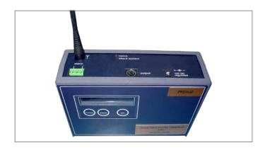
**AKC** is a radio-telemetric measuring system serving for wireless collection of temperature data in industrial conditions. It was designed for monitoring possible thermal runaway reactions in radioactive wastes processed by method of bitumenation but similarly it can be used for monitoring other reactive systems with thermal explosion risks in chemical industry.
